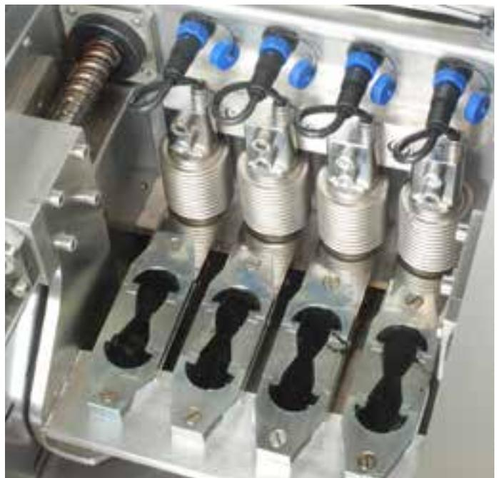
Detail of 81-PV10B02 and PV10C12 with four 81-PV10020 load cells and briquette moulds
