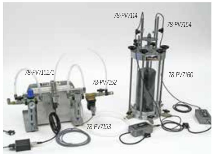
RM, Resilient modulus test set with 78-PV7160 cell
