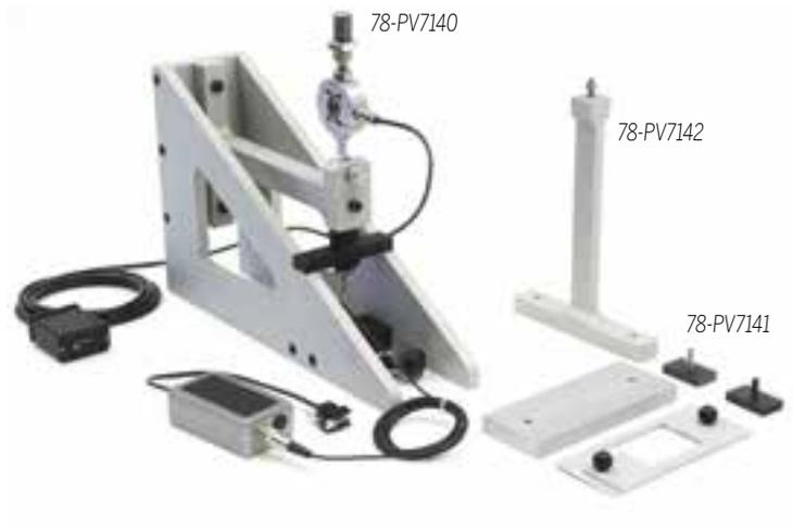
2PB, 2-Point bending test set
