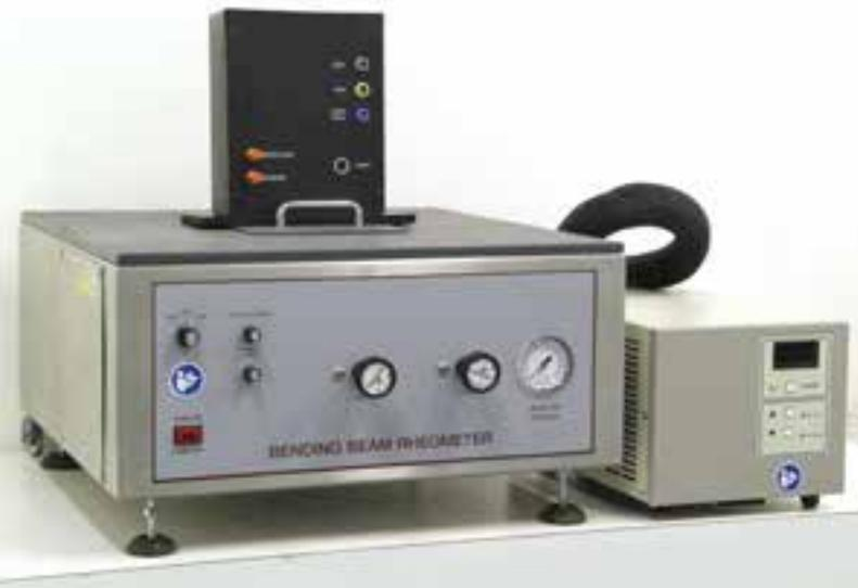
The BBR System consists of a fluid bath base unit, a three-point bending test apparatus which is easily removed from the base unit for specimen loading and unloading, an external cooling unit with temperature controller, and a calibration hardware kit with carrying case. The system includes the testing software.
