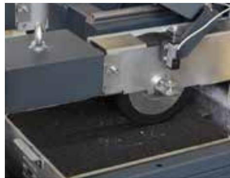
Asphalt slab 400 x 300 mm for EN 12697-22 tests
