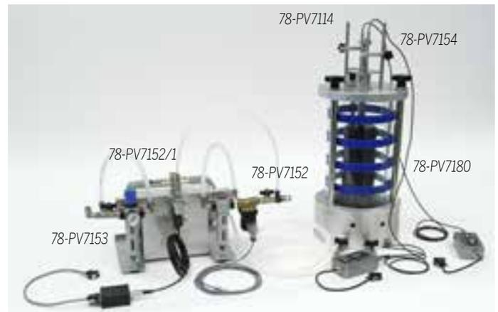
RM, Resilient modulus test set with 78-PV7180 cell
