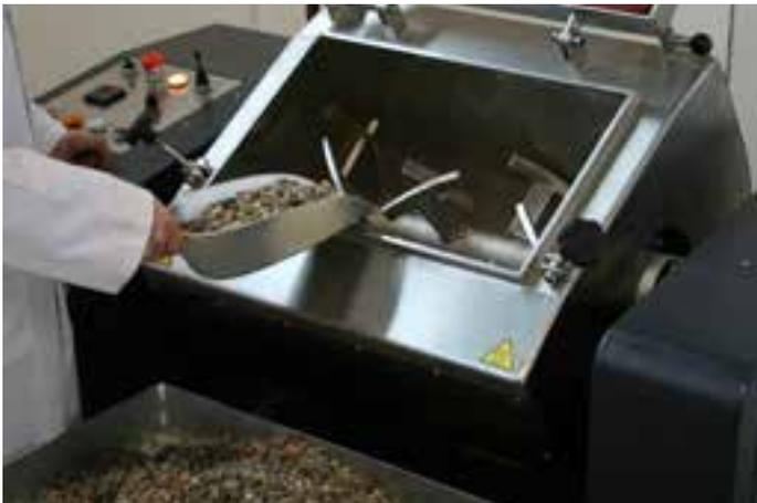
76-PV0077/B Detail of aggregate loading
