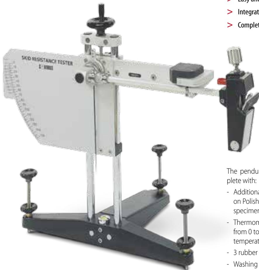
The apparatus consists of an adjustable pendulum arm and a spring loaded rubber slider (see accessories) mounted on the end of the arm. During operation the pendulum is raised and then allowed to swing freely, allowing the edge of the rubber slider to skid across the surface of the road or sample.
