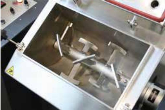
76-PV0077/B Detail of drum with helical mixing shaft
