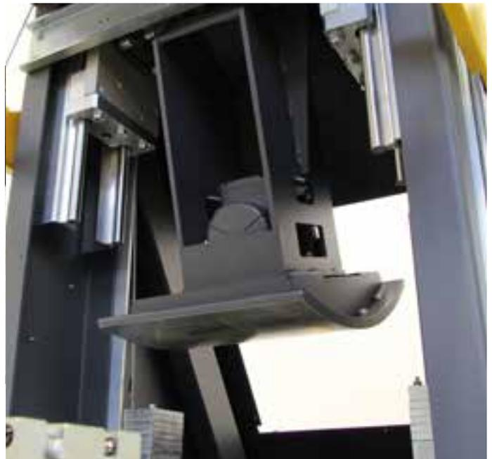
Detail of segment head incorporating vibration unit
