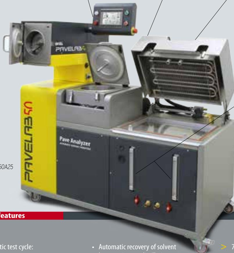
Level indicators are made of a high resistance material in order to be compatible with a **extensive range of solvents**.
