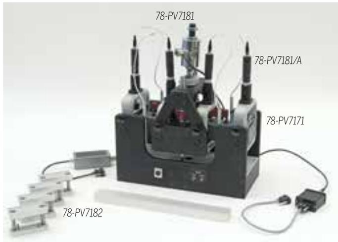
4PB, 4-Point Bending test set
