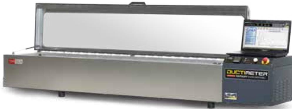
This research version further increases the high performance of the 81-PV10B02 model by more advanced specifications concerning temperature control, speed range and max. tension force, together with an extended use of stainless steel: frame, tank, cooling coil and
