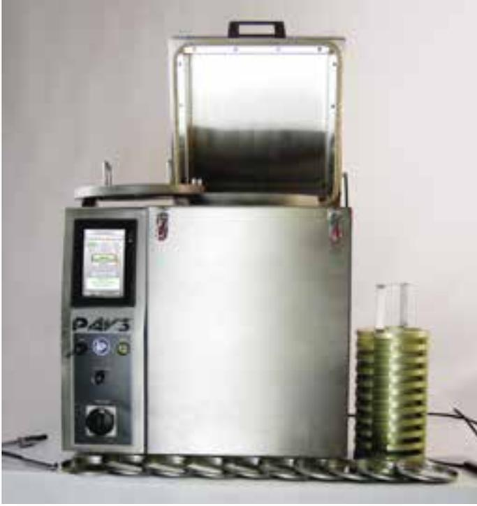
This apparatus is designed to simulate in-service oxidative aging of asphalt binder by exposure to elevated temperatures in a pressurized environment. This improved PAV model simplifies the running and documenting of asphalt binder aging operations.
