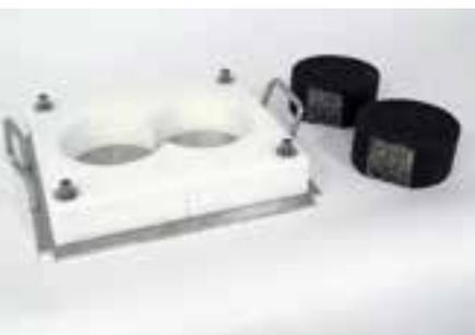
Tray with handles for double 150 mm diameter cylindrical samples
