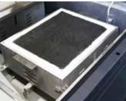
Asphalt slab 320x260 mm, mounted with plaster to AASHTO T324
