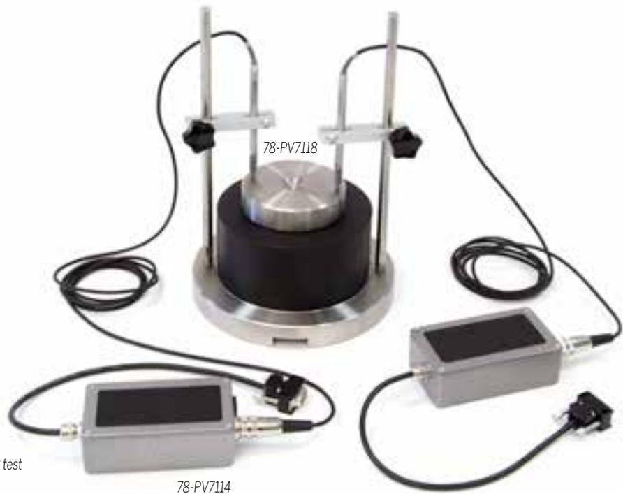
Set of accessories for UCC test to EN12697-25A test
