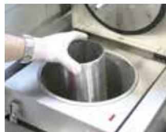
Placing the centrifuge cup into the centrifuge unit
