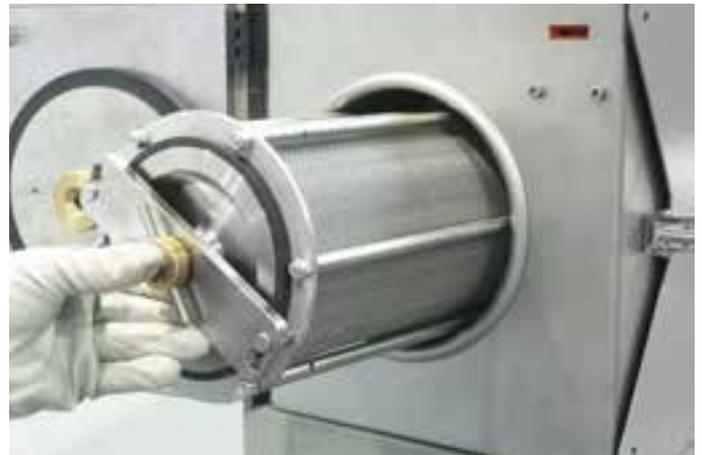
Placing the washing drum into the machine
