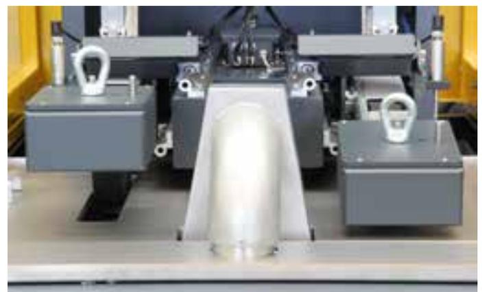
77-PV3UP10 Upgrading option. One of the two wheels is automatically lifted after test is completed continuing the test with the other wheel up to the rut target.
