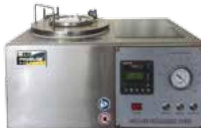
Stainless steel construction, holds up to 4 specimen containers, self contained automatic vacuum system, high precision controller featuring a digital display indicating time, temperature and the current stage of each process, maintains temperature up to 170° C with an accuracy of ±5°C.
