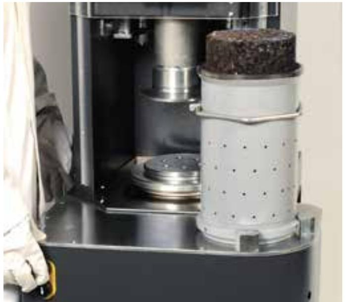
Integrated worktop with electromechanical extruder option 76-PV2520/15
