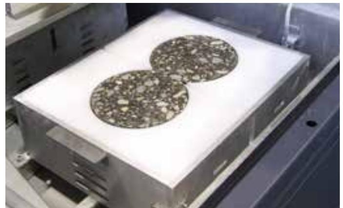
Mould adaptor for double 150 mm dia. Cylindrical samples to AASHTO T324
